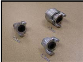
3/4 FNPT 2 lug fitting for 185's, 60 & 90 Lb breakers w safety pin.
